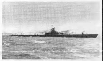
displacement 1475 (surf.), 2370 (subm.); length 307'; beam 27'; speed 20k (surf.), 8.75k (subm.); test depth 300'; armament 1-3"/50; 6-21" torpedo tubes fwd., 4-21" torpedo tubes aft.; complement. 6 officers - 54 enlisted men; class GATO
