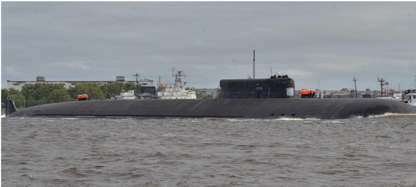
*The Belgorod sailing out from the shipyard in Severodvinsk for sea-trials in 2021. The vessel is built on the hull of what in the 1990s was supposed to become an Oscar-II class submarine. Photo: Sevmarsh*
