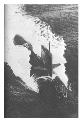
The <u>six boats</u> of Skipjack's design was based off of the successful Barbel class submarines that were based on the USS Albacore design.
