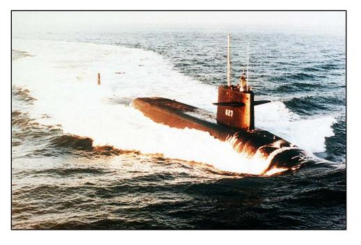
The James Madison <u>class</u> of 10 submarines were an evolutionary development from the Lafayette class of fleet ballistic missile submarine. They were identical to the Lafayettes except for being designed to carry the Polaris A-3 missile instead of the earlier A-2.
