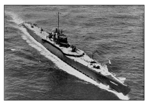
Originally, a small scouting seaplane was to be carried in a water-tight hangar abaft the conning tower. Two boats, in appearance and dimensions, Narwhal and Nautilus were similar to Argonaut and constituted "submarine cruiser" partially inspired by German success with long-range submarine in World War I.
