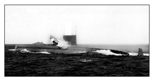
Begun as a dieselelectric submarine but completed with nuclear power, Halibut was the first submarine designed to launch guided missiles.
