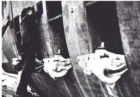
Collapsible hydrogen peroxide storage bags being removed from the 300-ton Type XVIIIB Walter boat U-1407 after the war. With the type of storage outside the pressure hull, fuel could be consumed without appreciable change in trim – seawater simply replaced the depleted volume.
